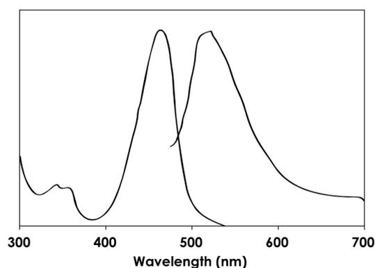
Fig. 1: Excitation and emission spectra for DeNovix dsDNA Ultra High Sensitivity Range quantitation reagent in the presence of excess dsDNA.
