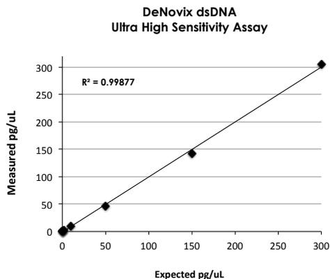
Fig. 2. Standard range using 10  $\mu$ L of sample in 200  $\mu$ L of dye reagent.
